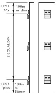
For a typical 2500x1220mm wide panel, customers mount the continuous lengths along the wall at 3 different heights parallel with the floor. These are secured to framing at 400mm on center or to blocking at 200mm on center.
